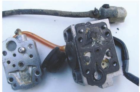
These are the pipes & carburettor from a Mantis tiller that had petrol left in it for over a year. This was so bad it had to have new pipes, filter and a new carb.
